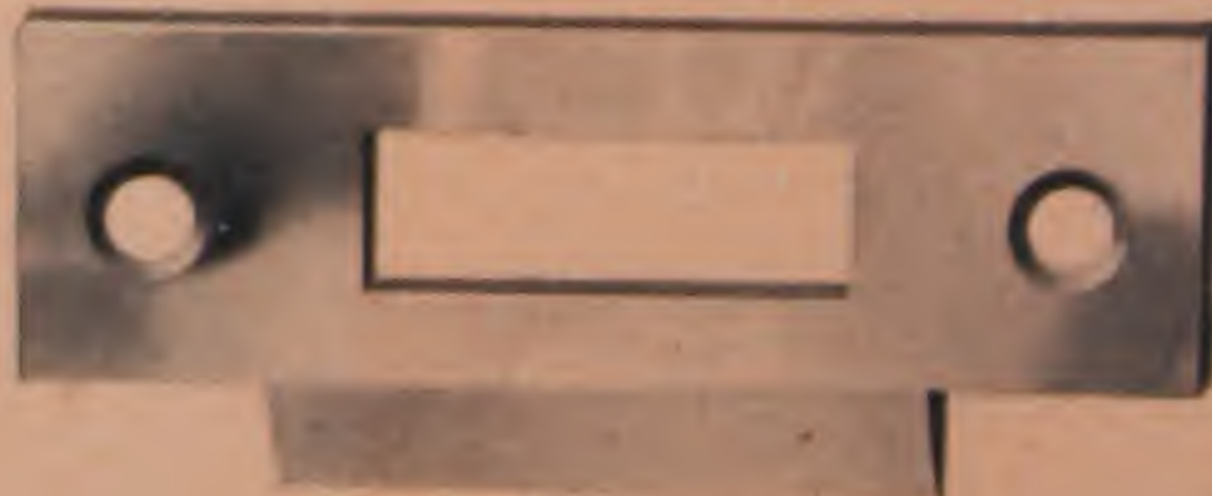
No. 330A— 2\frac{1}{4} " x 1\frac{1}{4} ". Lip Projects \frac{1}{8} ". Slot, \frac{1}{8} " x \frac{1}{8} ". Countersunk for No. 4 Screws.
